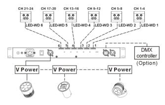
Note: You can set the DMX address of the fixtures connected to the output (like V Power show above) from 1-4, 5-8, 9-12, 13-16,17-20 or 21-24 according to your needs.
