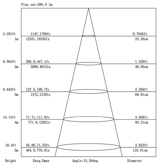
Note: The curves indicate the illuminated area and the average illumination when the luminaires at different distance
